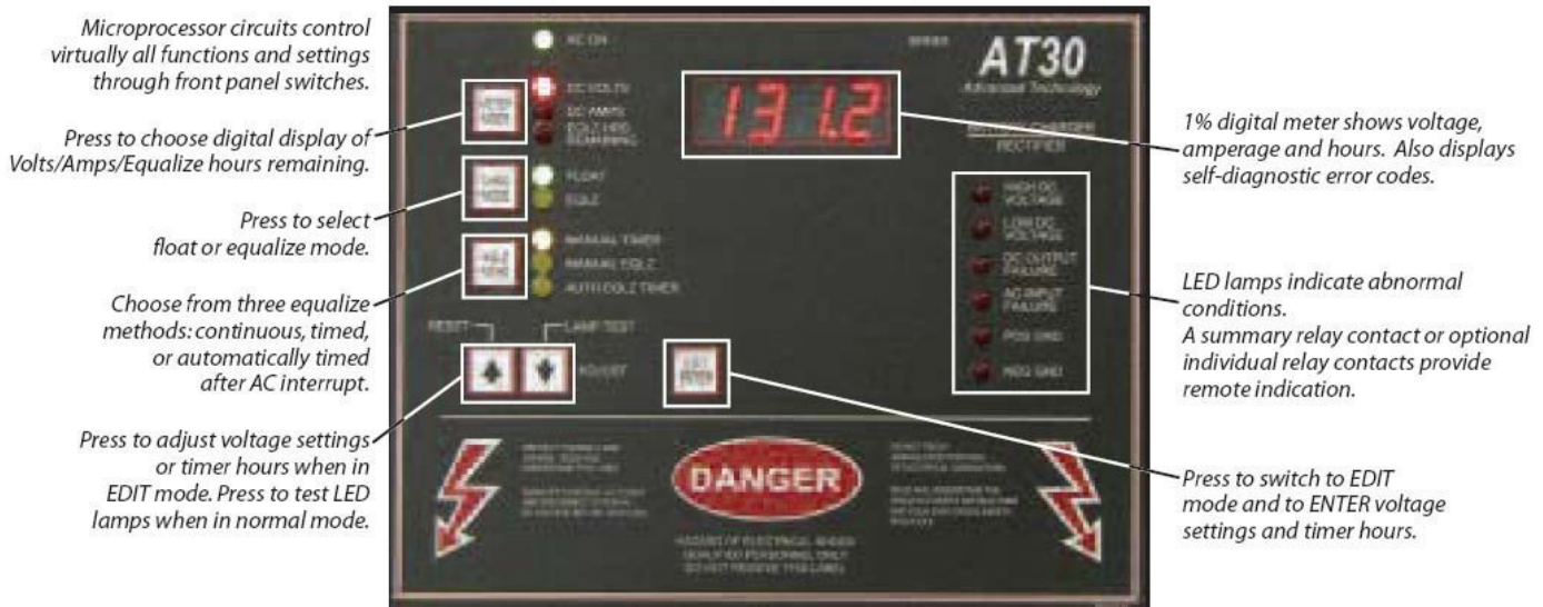
Critical adjustments can be disabled for tamper proof operation.
